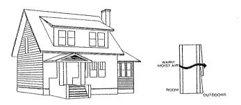
Today's homes are much "tighter." Windows and doors are built to reduce air leakage substantially. Weatherstripping, modern insulation, vapor barriers, and construction techniques intended to keep out cold air all can lock moisture inside. As a result, moisture created by bathrooms, kitchens, laundries, and occupants no longer flows to the outside, unless provisions for mechanical ventilation have been made. So it's very easy to build up excessive, even harmful, moisture levels in today's homes.
